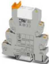
PLC-INTERFACE, consisting of PLC-BPT.../21-21 basic terminal block with Push-in connection and plug-in miniature relay with multi-layer gold contact, for mounting on DIN rail NS 35/7,5, 2 changeover contacts, input voltage 12 V DC
